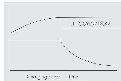
For the charging itself it is not important if the battery is partly or completely discharged. The battery can stay connected to the charger for a long period, the surrounding temperature should be in the range of –25°C to 40°C. In case the battery has been connected to the charger with the wrong polarity then this will be indicated through a red light („Verpol“). Disconnect the battery from the charger immediately.
