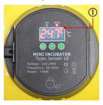
On the control panel left outer corner there is the connection for the electricity plug. It is important to push the plug in well to allow the incubator to function properly. As soon as the plug is connected, the incubator will turn on.
