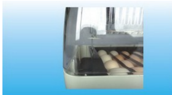
Fig. 4: pay attention that there's an egg turning rod in the transparent case at the upper part of device. The rod must insert into the channel of egg tray for the egg turning. The egg turning motor runs as long as the device is powered on. It runs one cycle every four hours so that it's very slow. The egg is turned once about every 4 hours.
