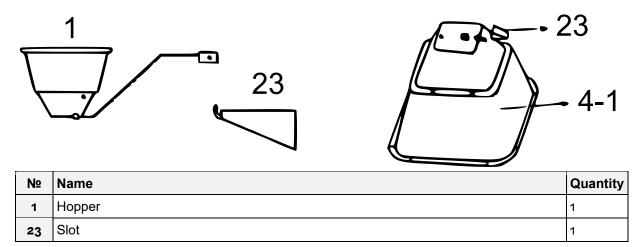
Turn the hopper (1) upside down and push the slot (23) completely into the guide channel on the underside of the hopper.
