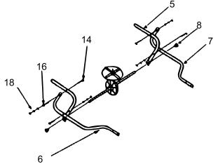
Fasten the rear hopper supports (5) to the right hopper support (6) and the left hopper support (7), using the M6×50 screw (14), small washer (16) and hexagon nut (18) as shown in the figure above.
