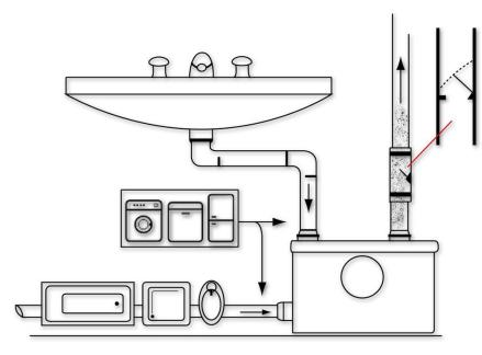
For the lifting system to switch on when the sewage water is evacuated, the incoming sewage water line should have a gradient of at least 2-3 % and a height difference of at least 20 cm from the siphon to the entrance to the macerator.
