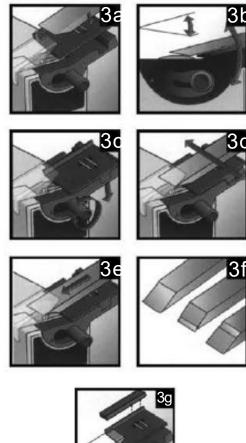
Grinds bits and chisels up to a width of 50 mm (2").
