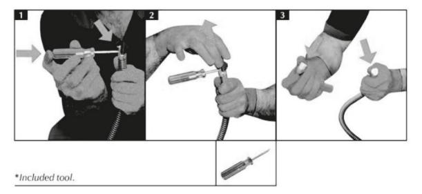
• To be able to use the pipe cleaning device, the white plastic sleeve must be inserted correctly. Please check the seat of the sleeve before each use (2). Make sure that the lever is in pos. 4a, and push the spiral through the device until the drill comes out of the device at the front.
