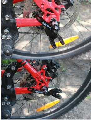
Open the quick clamp and remove the opposite nut and spring. Hold the lever and pull out the axle and spring. Remove the complete axle, but make sure that the wheel stays in place.
