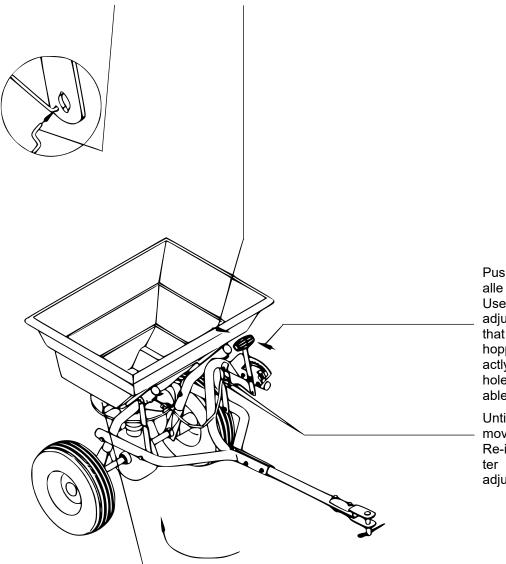
Push the handle alle the way down. Use it to adjust the adjustable plate so that the hole on the hopper bottom exactly matches the holes on the adjustable plate.
