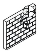
2. Drill the holes marked and fix the wall bracket to the wall with the provided bolts.
