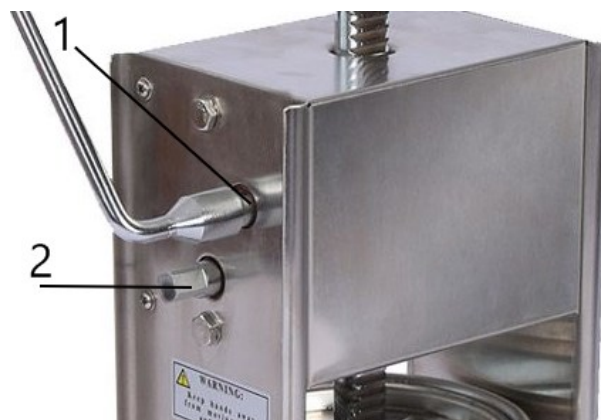
(1) Fast gear shaft; (2) Slow gear shaft
