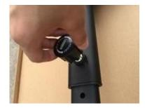
5. Adjust the seat scooter mount to the size of your board and secure the setting with the screws. Use the spanner (5) for this. Now fix the board with the supplied fabric straps with Velcro. Make sure that the go-kart is held firmly in place. Only use the kart with your board if it can be mounted appropriately.
