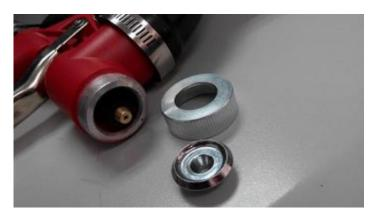
3. Fix the connection tube to the casing with the help of the clamp and screw delivered.
