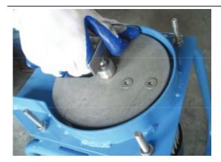
Remove the rotating plate fixing the cutter plate. Then take the cutter plate (10) from the base plate (15) and clean it.
