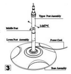
3) Join the Heating Element Assembly (1) and the Upper Post Assembly (7) together, then fix them tightly by rotating the Knob, and put the power cord supply into the clamp.
