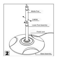
Join the Lower Post Assembly and the Middle Post (9) together with 3-M5X6 screw.
