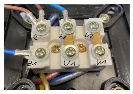
For there are different configurations of the cables, you will need to check, before changing the direction of rotation, if the configuration of colours in the motor is as follows:
