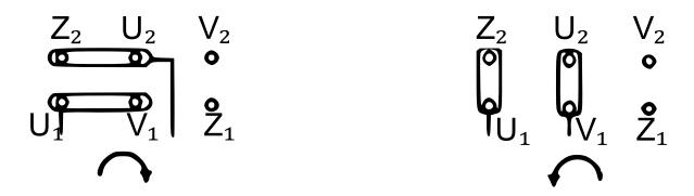
**Note:** The direction of the point is displayed to show the rotational direction from the shaft end.
