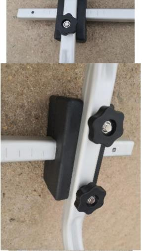
5. Adjust the clamping block on the axle sleeve. The scales on the axle sleeve can help. Tighten the knobs on both clamping blocks.
