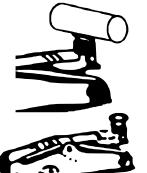
Always place the load in the centre of the support surface of the jack so that it rests as securely as possible.
