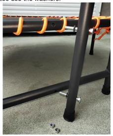
5. Insert the second part of the base tube and fix it with the knurled screw.
