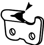
Keep all the chain links equal. Start with the link with the most damage and file all the links back evenly.
