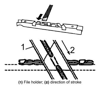
**Notice!** If the surface of the top panels or side panels is damaged, file them back until the damaged area is removed.
