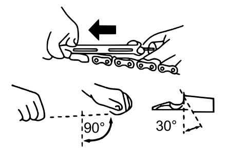
First sharpen the links on one side of the chain. File each link from the inside to the outside. Then turn the saw over and repeat the process for the links on the other side of the chain.
