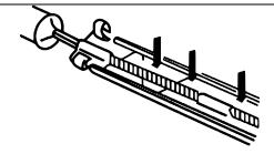
4. Make sure that the file is firmly seated in the guide groove.
