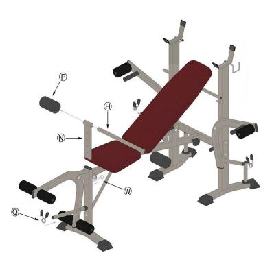
Insert the long bar (with foam cap) **(H)** into the adjustment lever **(N)**. Then slide one large foam cap **(P)** on either end of the long bar. Set the entire assembly **(H, N, O)** into the front support and secure it with the ring pin **(W)**. Finally, set the spring clamps **(Q)** in as shown.
