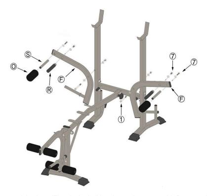
Attach the side bent training bars (F) to the barbell brackets using screws (1). Pay attention to the correct orientation of the F bar (arrow). Insert the handles (R) and the grip levers (S) into the large holes of the side bent training bars and fix them using screws (7). Slide one small foam cap (O) on either grip lever (S).
