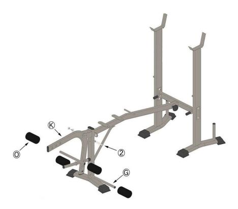
Connect the front bent training bar **(K)** with the front support using screws **(2)**. Slide the small lever (with foam) **(G)** through the hole (see fig.) and cover the ends of the small lever **(G)** using a small foam cap **(O)** on either end.
