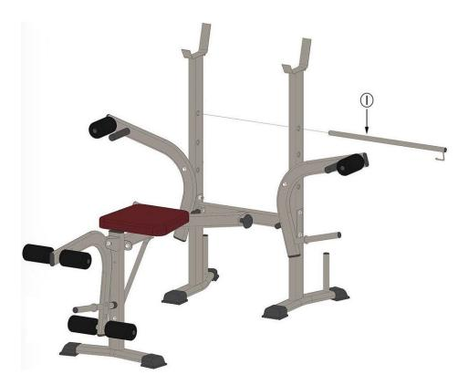
Insert the back rest lever (I) through the corresponding holes of the barbell brackets (see fig.).
