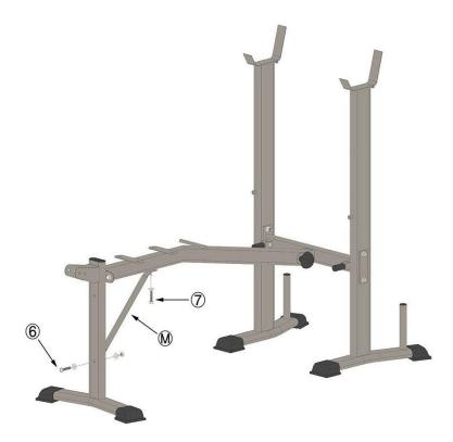
Connect the main rod and front support with the support bar (M) using screws (6) and screws (7).
