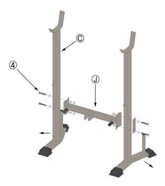
With screws (4), connect the barbell bracket (C) and connection rod (J).
