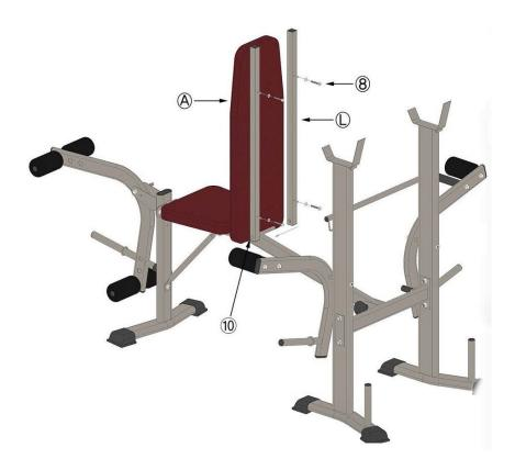
Fix the back rest support bars (L) to the main rod using screws (10), attach the back rest (A) to the back rest support bars and secure it with screws (8).
