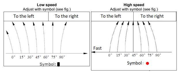
The user can select the appropriate nozzle orientation for different pool types, e.g., a low speed with a large radius of movement, by setting the circle symbol O to the 45° position (movement to the left) or 75° position (movement to the right).
