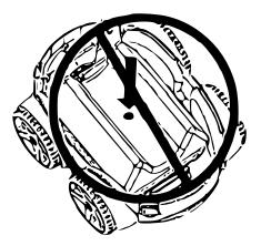
• Do not lift both sides of the filter unit at the same time.
