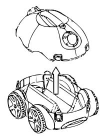
2. On one side, press down the bracket and lift the filter unit.
