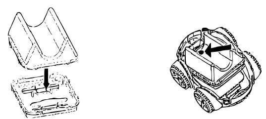
Press down the bracket on the opposite and correctly place the filter unit.
