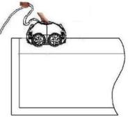
2. Hold the cable until the robot has filled itself with water and begins to sink towards the floor.
