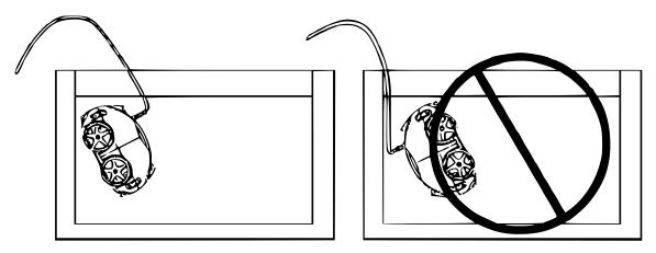
• Store the cleaning robot on a flat surface. No hard objects must touch the casing of the robot to avoid damage.
