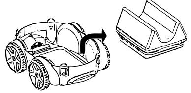
4. Open the small bracket and take out the filter bag for cleaning.
