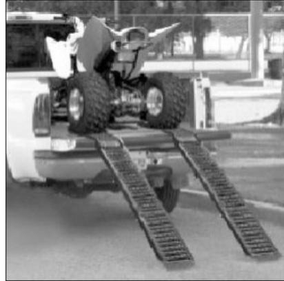
**Step 2:** To use the product for ATVs/quads, remove the stop and open the 2 parts as shown.
