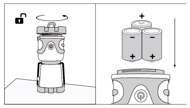
1. Turn the lamp upside down and unlock the base2. Insert the batteries in the correct direction. Cauby turning it.by turning it.tion: Do not use rechargeable batteries!
