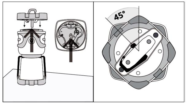
3. Replace the base while making sure that the pin 4. Re-lock the base by turning it. is at the correct position (see arrow).
