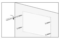
4. Cover the open holes with the rubber plugs.
