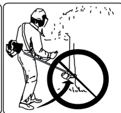
Do not cut down trees that are too thick!
