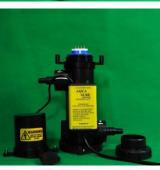
Fig. 6 Insert the new lamp and a new O-ring.
